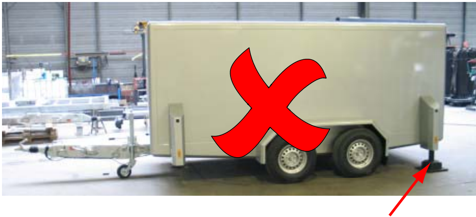
Image 1-1 Wrong way to level trailer
