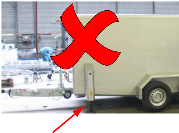
Image 1-2 Wrong way to level trailer
